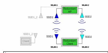
m igtarrowWLANs with same color must have identical RF type, SSID, and security settings
