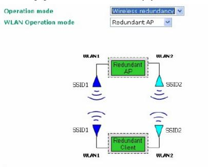
The following figure shows the Wireless Redundancy operation mode:
